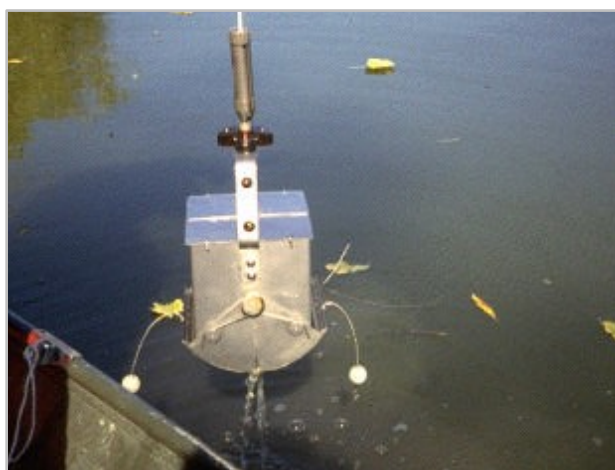
Ekman Dredge Grab sampler – typically used in deep waters and lakes. Ponar Dredge Grab samplers are also used in deep waters and lakes.
