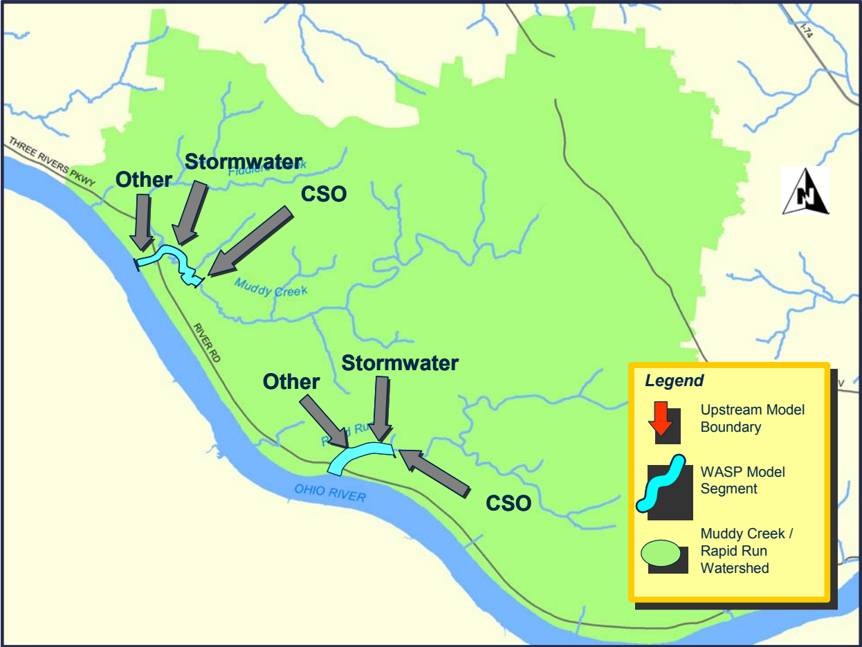
Exhibit 3: Figure 4 Conceptual Muddy Creek/Rapid Run WASP Model
